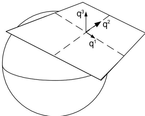
**Fig.2: Tangent plane at a curved surface**
