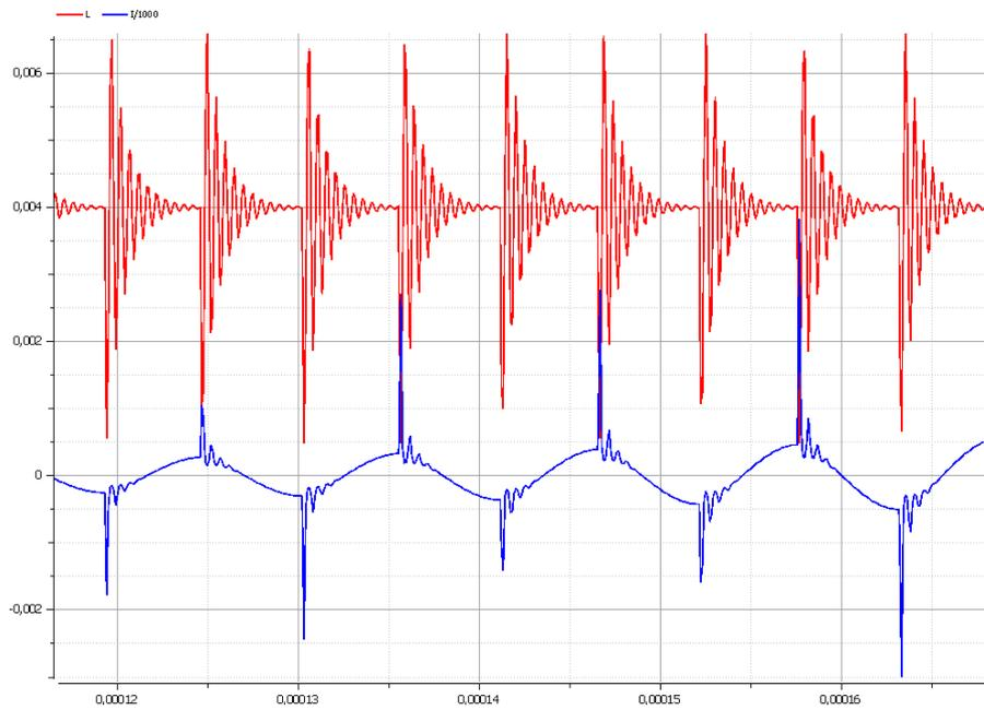
Figure 3: Variable inductance  $L$  and current  $I$  in an enlarged time slot.
