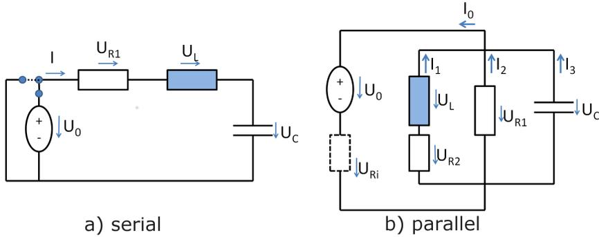
Figure 1: Serial (a) and parallel (b) resonance circuit.
