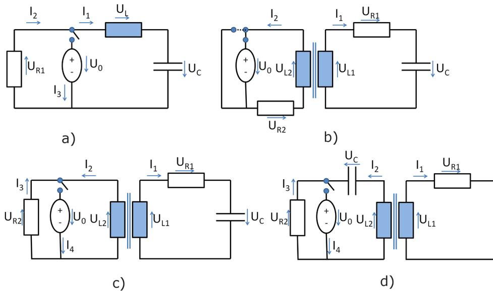
Figure 8: Variants of the parametric oscillator circuit. a) source position modified, b) inductive coupling for Fig. 1a, c) inductive coupling for (a), d) oscillator completely in primary circuit.
