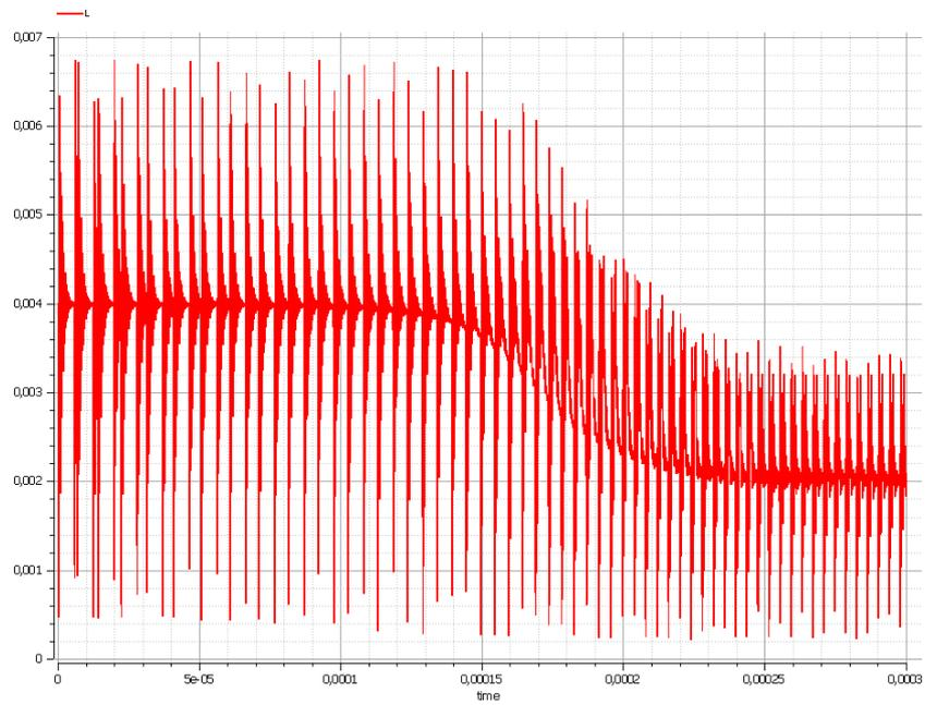
Figure 6: Saturation effect of inductance  $L$  over time.
