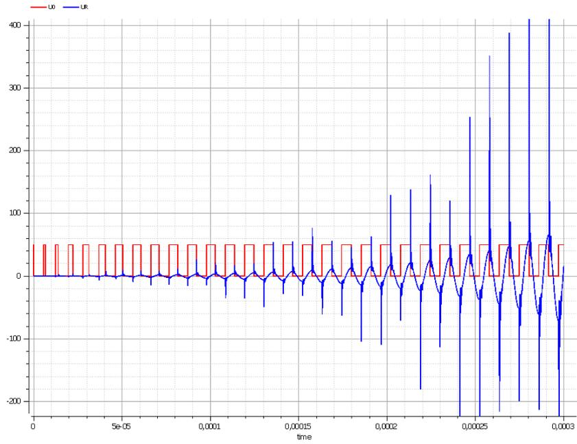
Figure 2: Switched voltage source  $U_0$  and voltage at ohmic resistance  $U_R$  in the serial parametric oscillator.
